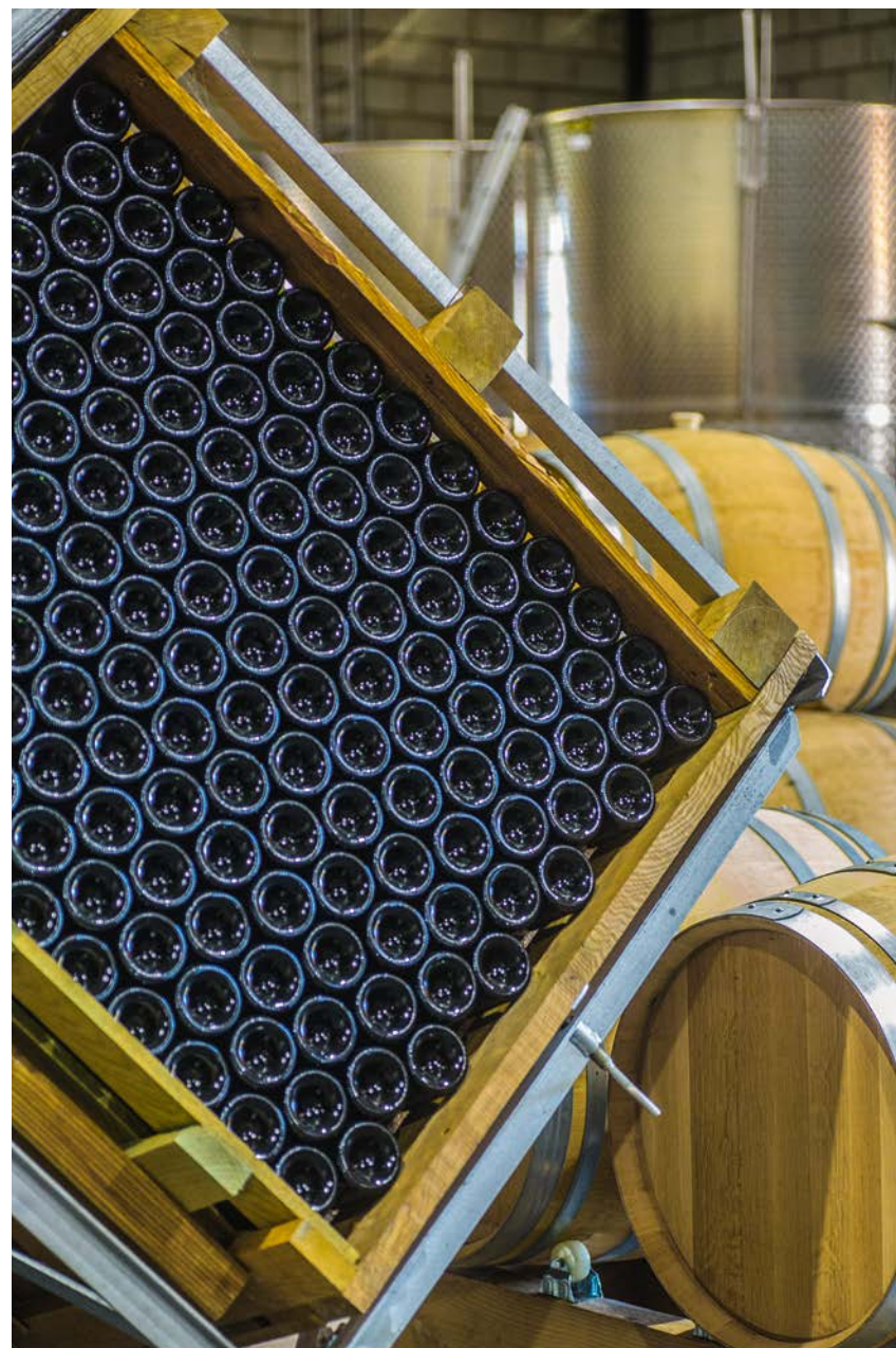
After the maturation "sur latte" follows the remuage with double gyro pallets, in order to bring the lees to the neck of the bottle.
